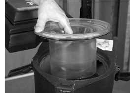
Remove the separator assembly to clean the vacuum cone.
