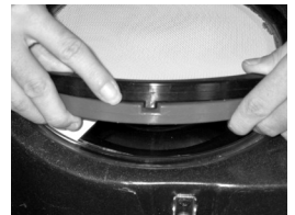
The upper secondary filter (black) fits on the primary filter.
