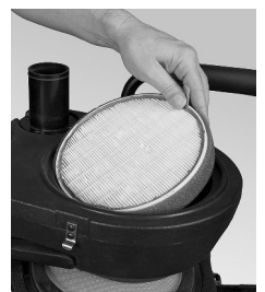
Insert the HEPA-type filter in the lid with the small tab facing you.
