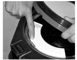
Match the rectangular notch on the lower primary filter (burnt orange) with the filter housing.
